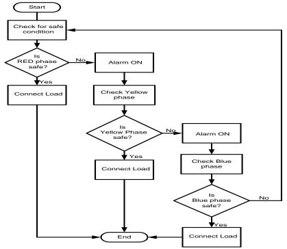
Figure 4: Flowchart of the automatic power selection switch
