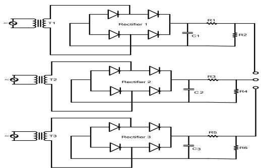
Figure 2: A Three-Phase Power Supply Unit
